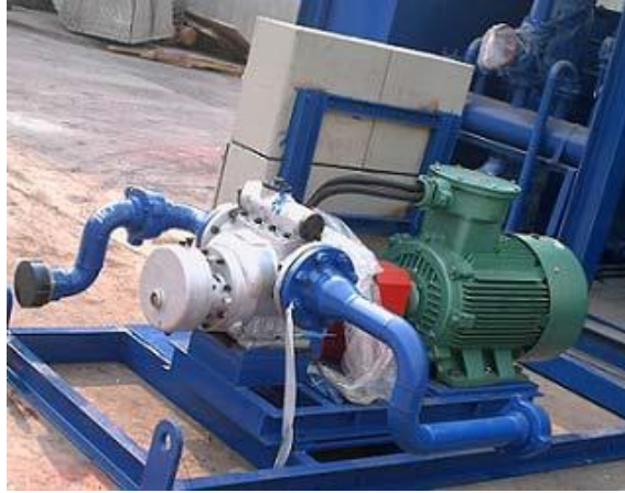
Figure 173 Crude oil transfer pumps
