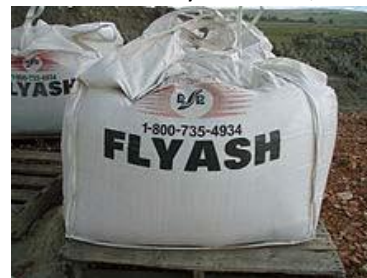
Figure 3 Fly Ash Absorbent for Fluids in Mud Pits
