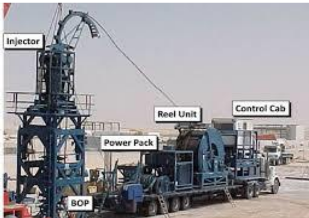
Figure 140 Coiled tubing unit
