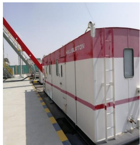
Figure 11 Mud logging unit
