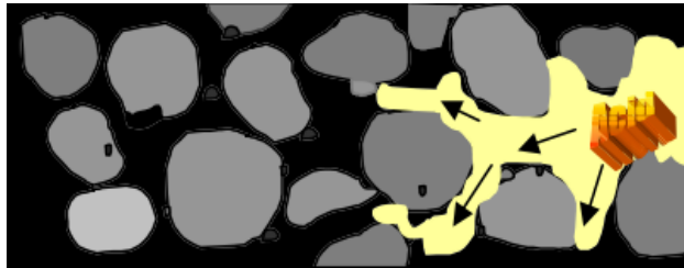
Figure 151 Acid reaction enlarges pore spaces
